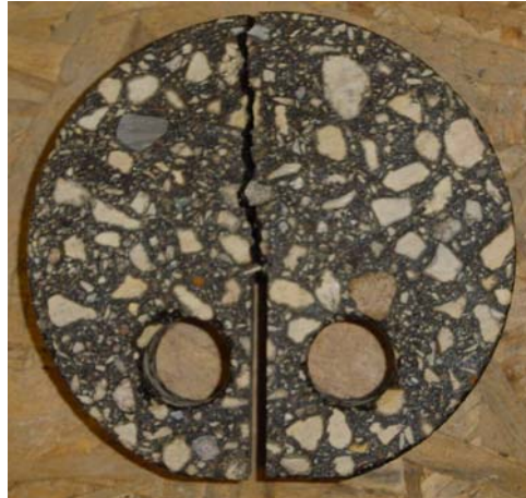
Figure 6.3. DC(T) specimen after testing
