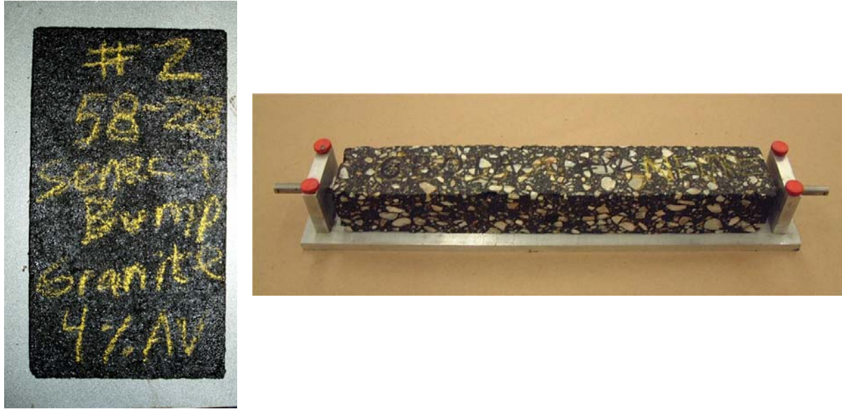
Figure 6.23. Received sample (left) and beam specimen prepared for testing (right)
