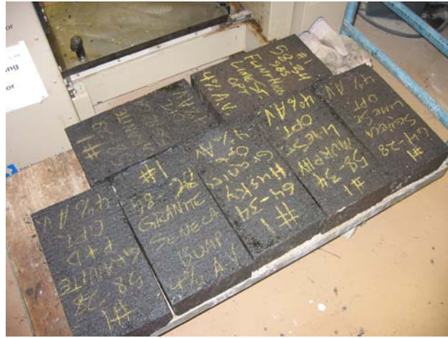
Figure 6.16. Compacted slabs before cutting
