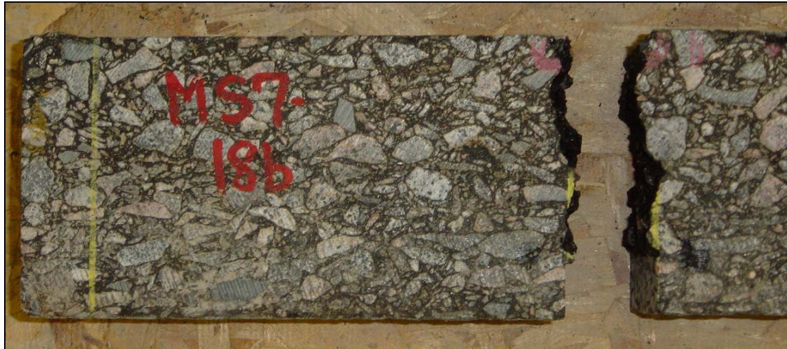
Figure 6.15. SE(B) specimen after testing
