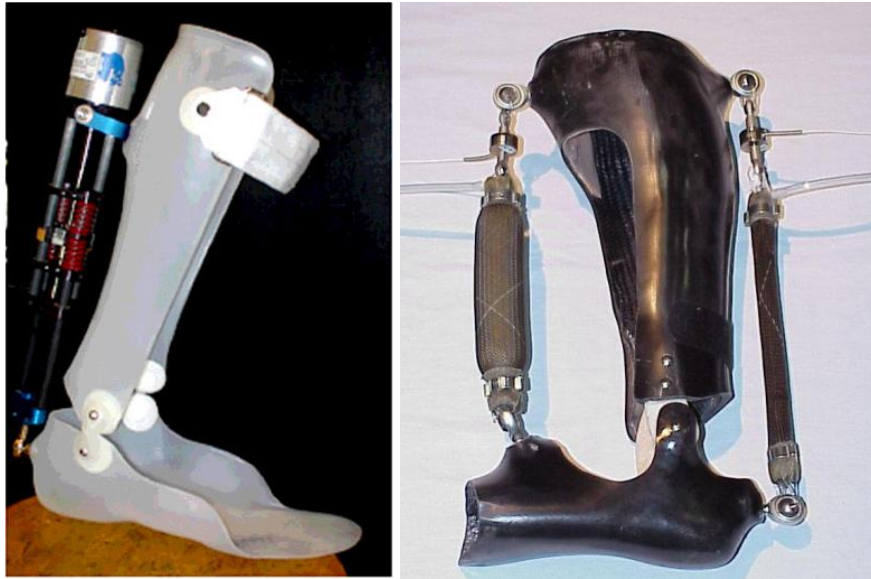
Figure 6. AFO using SEA by MIT (left) and powered AFO using PMA by University of Michigan (right).
