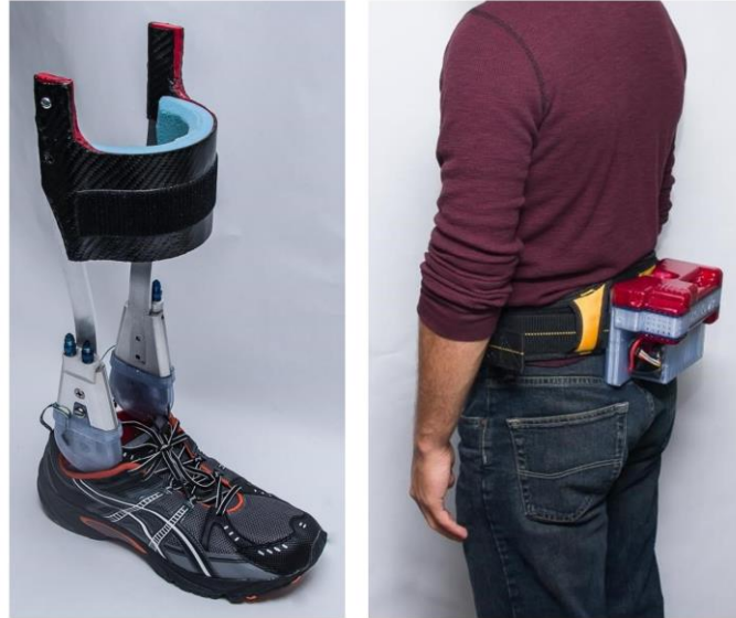
Figure 2. Hydraulic Ankle-Foot Orthosis (HAFO) developed by University of Minnesota.
