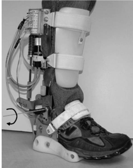
Figure 7. Powered AFO using robotic tendon technology.
