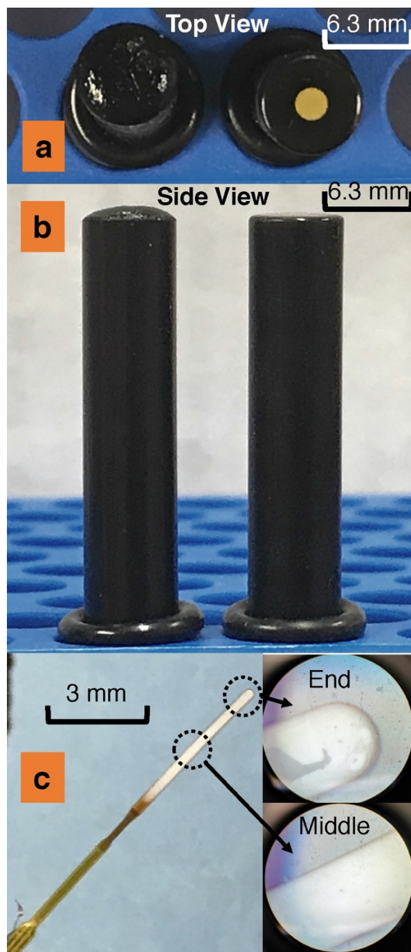
Figure 4.5 (a) Top and (b) side views of thick membranes (200 \mu\text{m} thickness) with a CIM carbon solid contact (left) and spin-coated thin-layer membranes (30 \mu\text{m} thickness, translucent yellow) without CIM carbon solid contact (right); (c) dip-coated membrane on a microelectrode, along with microscope views.
