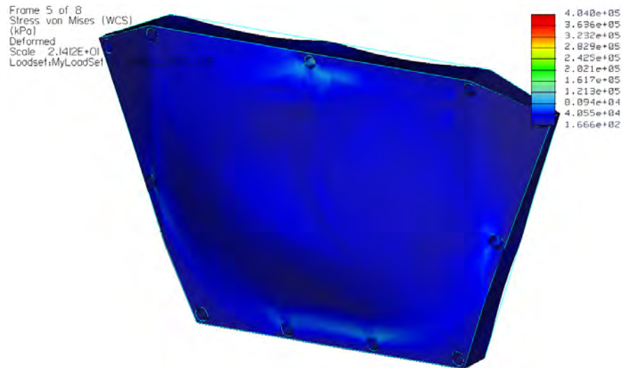
Figure 4.12: FEA Analysis of Shell Deformation
