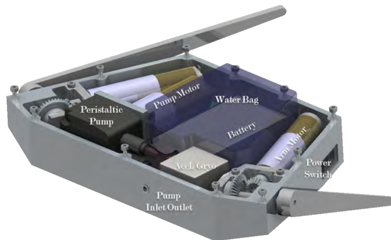
Figure 3.14: New Design with Labeled Components
