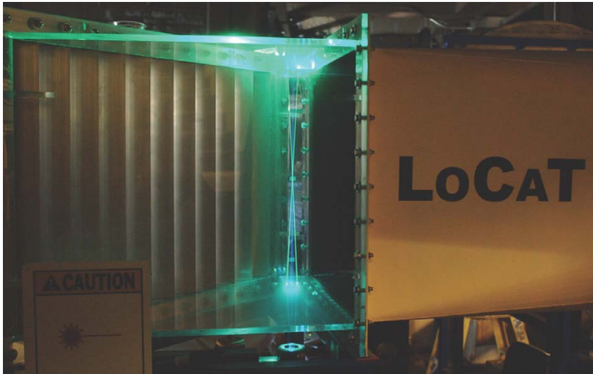
Figure 36. LDV measurements in corner #1, after turning vanes in plane of symmetry, z/W = 0 .
