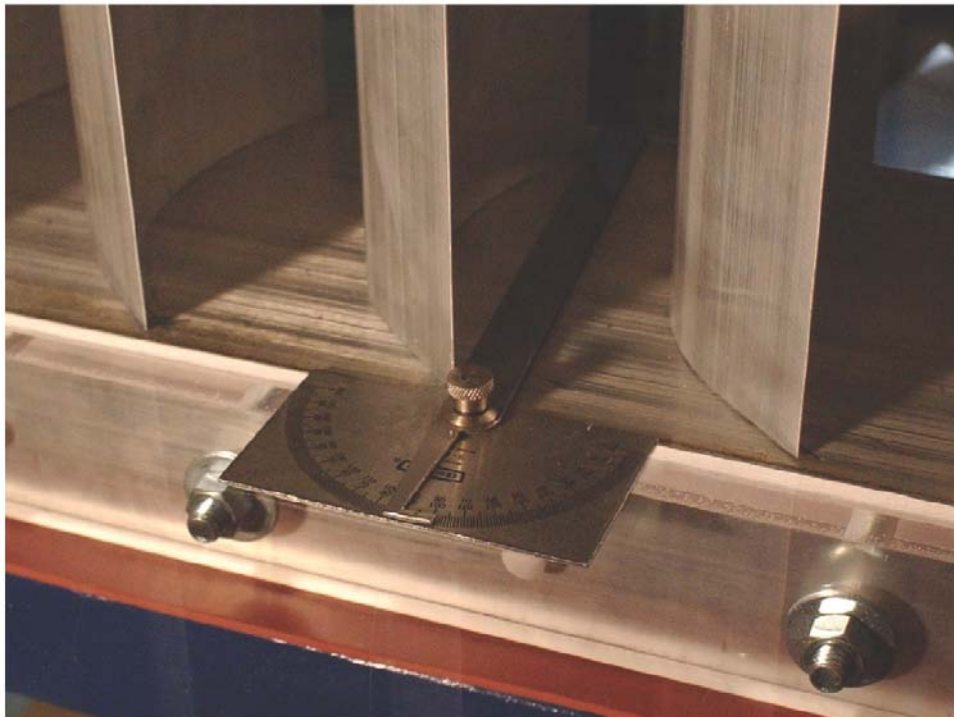
Figure 11. Experimentally verifiable (measurable) angles on the installed turning vanes, here illustrated on corner #1. Angle \alpha was measured with a machinist's protractor.
