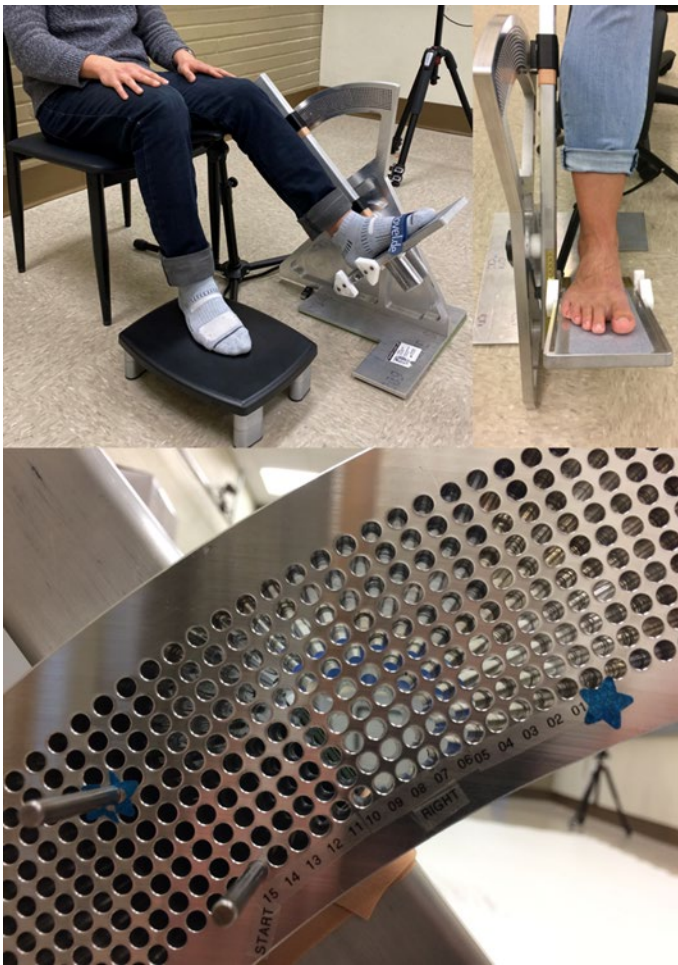
Figure 3-1. Ankle proprioceptive acuity system (APAS). (Top) Experimental set up. The examiner adjusts the leg rest and footrest to align the ankle with the system center of rotation before starting the testing procedure. (Bottom) A subset of holes in the pegboard. Each hole in the vertical direction indicates as 0.1 -degree difference in angle and in horizontal direction illustrates a 1 -degree difference. Stoppers are inserted to a specific hole to identify the initial and target locations of ankle position.
