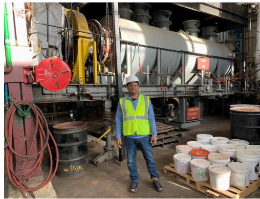
Sunil Tripathy stands by NRRI's pilot scale biomass conversion kiln at NRRI Coleraine.
