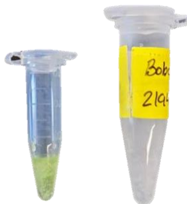
Figure 6.5. Visual Comparison of Bobcat339. 50 mM Bobcat339 in DMSO from MedKoo (left) and house-synthesized (right)
