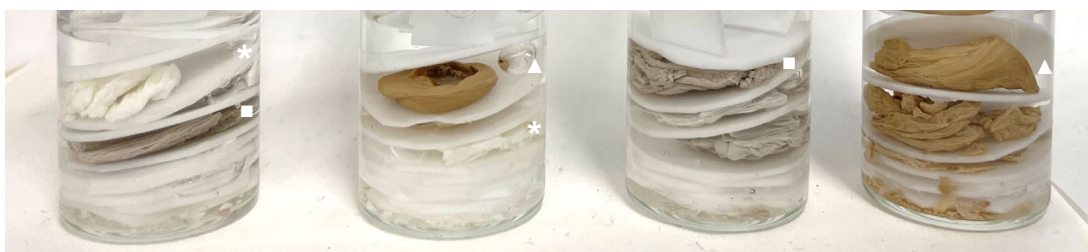
Figure S2.4. PHIL-IONP coprecipitates in water after 6 months. PHIL without IONPs is white (■), increasing concentration of sIONP results in darker tan color (▲), increasing concentration of EMG308 results in darker grey color (*). Fragmentation of precipitate is due to sample transport knocking tablets against glass. Tablets with more sIONPs are less fragmented. Solution remains clear indicating IONPs are not leaking.
