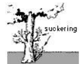
Figure 13. Suckering is one symptom of construction damage.
