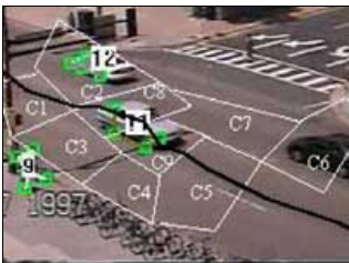
The traffic data processor divides a video scene into multiple cells to track vehicle movements.
