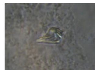
Figure 4. Example of protein crystal that constitutes a partial crystallization success. Crystallization conditions: 15% PEG 1050, 3 µg protein, and 0.1M sodium citrate at pH 5.6.
