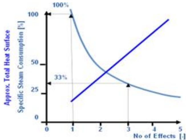
Figure 11: Steam consumption VS Number of effects (Source: GEA Group AG, 2013)
