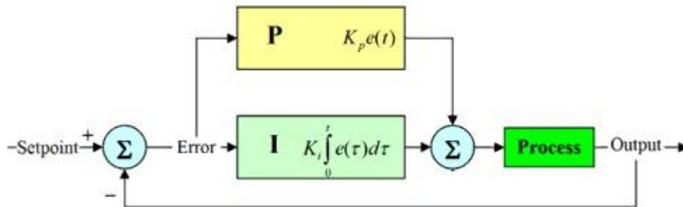
Figure 23: PI Controller (Source: University of Washington, 2013)
