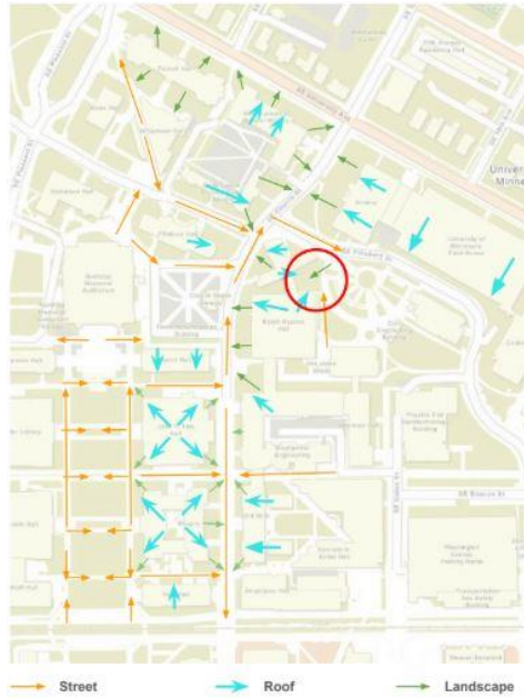
Figure 26: Water flow on site
