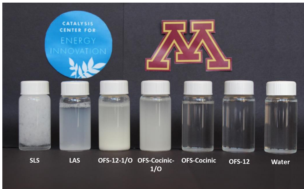
Figure 4-25. Surfactant solutions after addition of \text{CaCl}_2 (Surfactant concentration: 2 \times \text{CMC} , Concentration of \text{CaCl}_2 : 50,000 ppm) Note: Image taken after two weeks of making the solution
