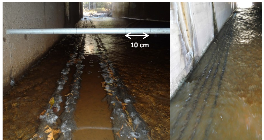
Figure 1. Testing plastic mussel spat rope in a Minnesota culvert during low and low-moderate flows. (Kozarek and Hernick 2018). This product functions as desired but is composed entirely of plastic fibers, easily shedding microplastics.
