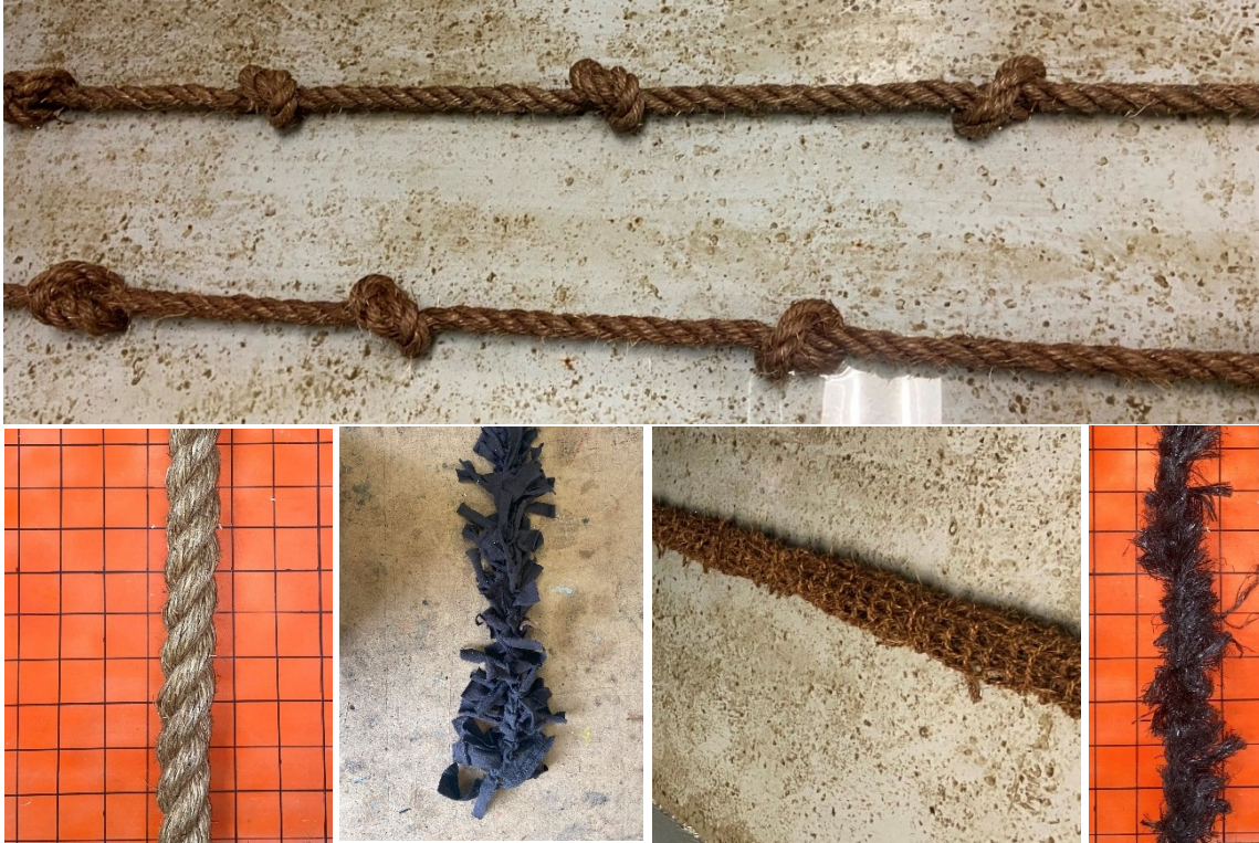
Figure 9. Examples of different prototype rope retrofit configurations tested in the flume.
