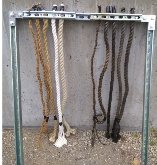
Figure 2. Ropes before placement in the water. From left to right are untreated coir, manila, sisal, cotton, and hemp, then the same sequence treated with pine tar. The near side of the frame was placed downward in the water
