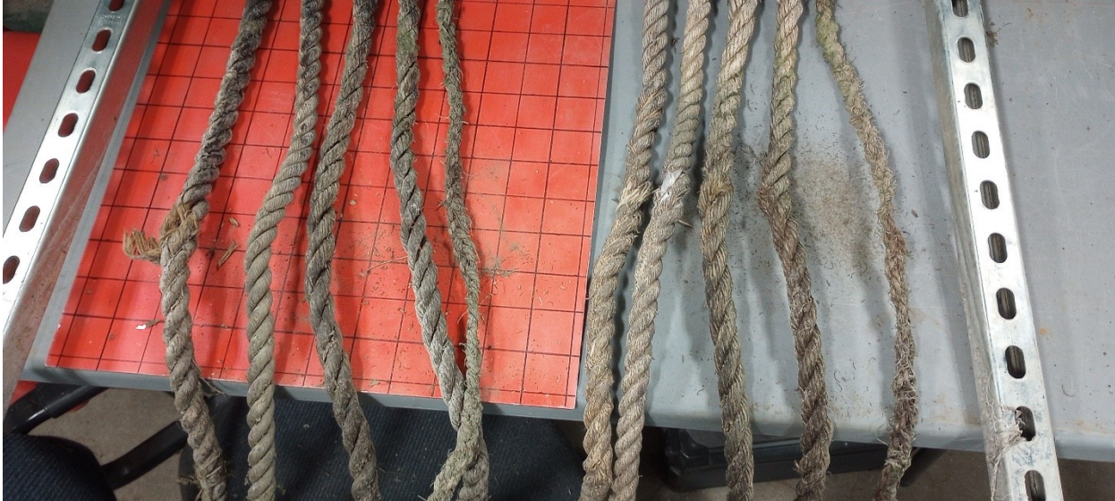
Figure 4. Ropes after drying. From left to right, untreated hemp, cotton, sisal, manila, and coir, then the same sequence treated with pine tar. Ropes were evaluated by manually twisting at mid-length.
