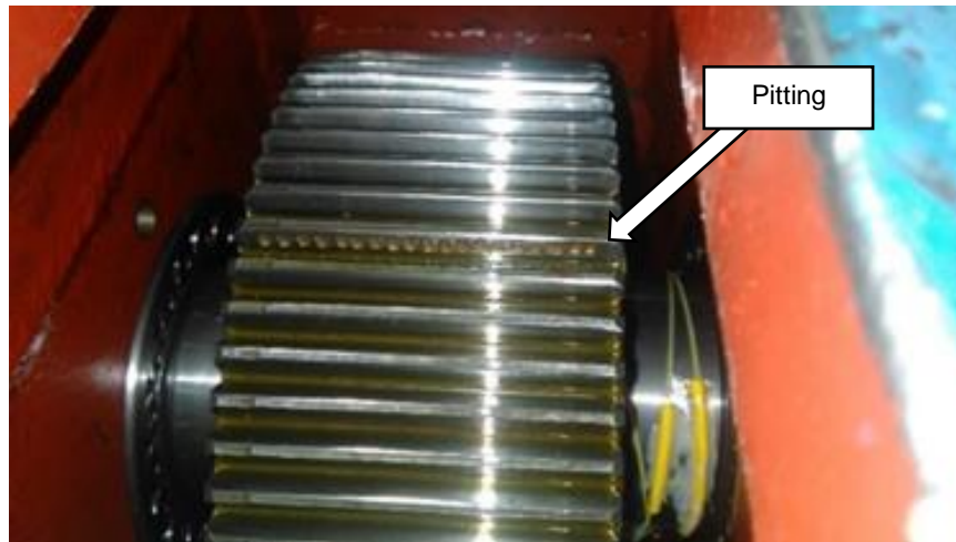
Figure 14: Single pitted gear tooth
