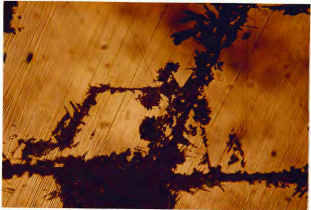
Figure 39. Photomicrograph of bluish covelite and dark gray chalcocite in galena (yellow). Crossed polars. Field of view: 2.2 x 1.5 mm.
