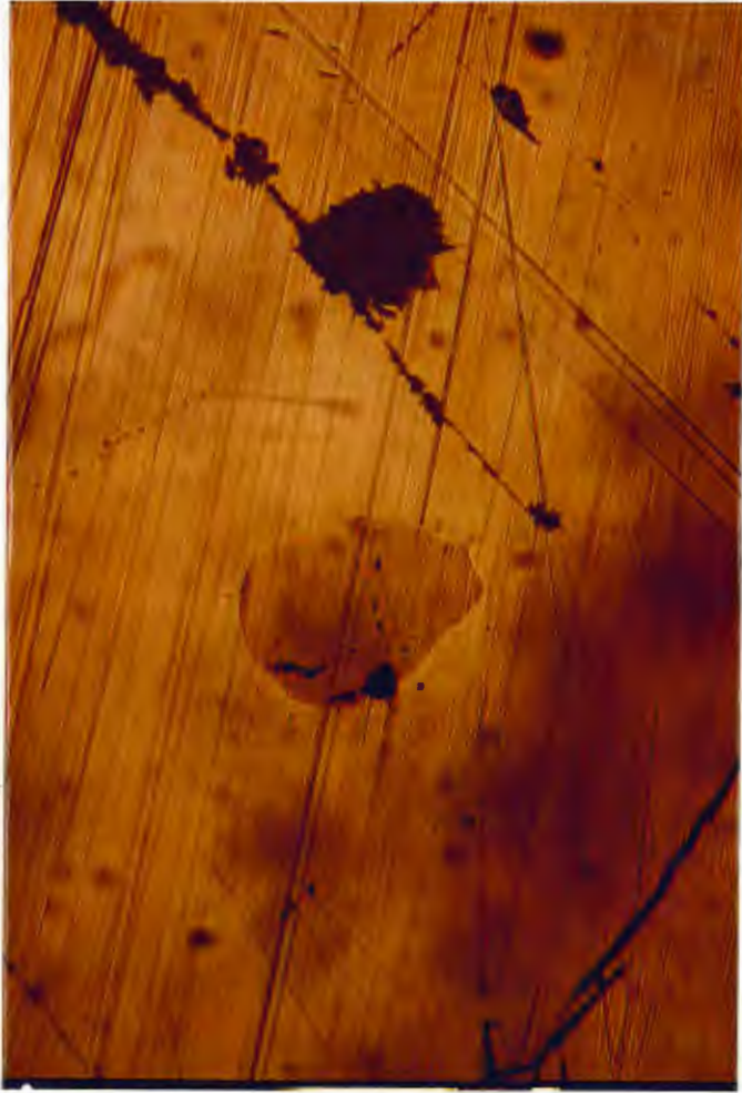
Figure 35. Photomicrograph of gray tetrahedrite exsolution bleb in galena. Crossed polars. Field of view: 1.5 x 2.2 mm.
