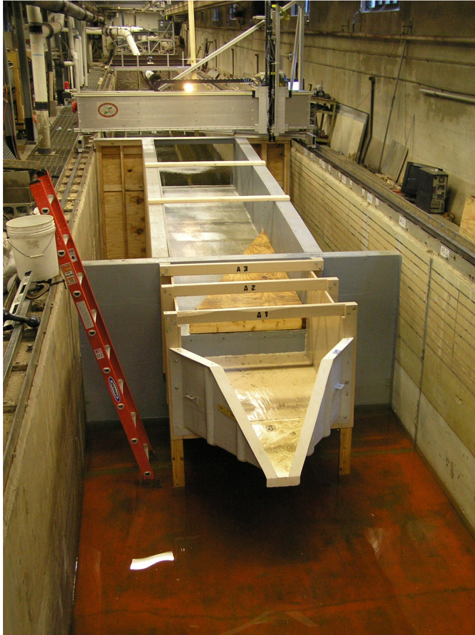
Figure 5. Image of test setup in Main Channel with the 4 foot approach section and 2 foot H Flume attached at downstream end, recessed from the approach slope by 35%.
