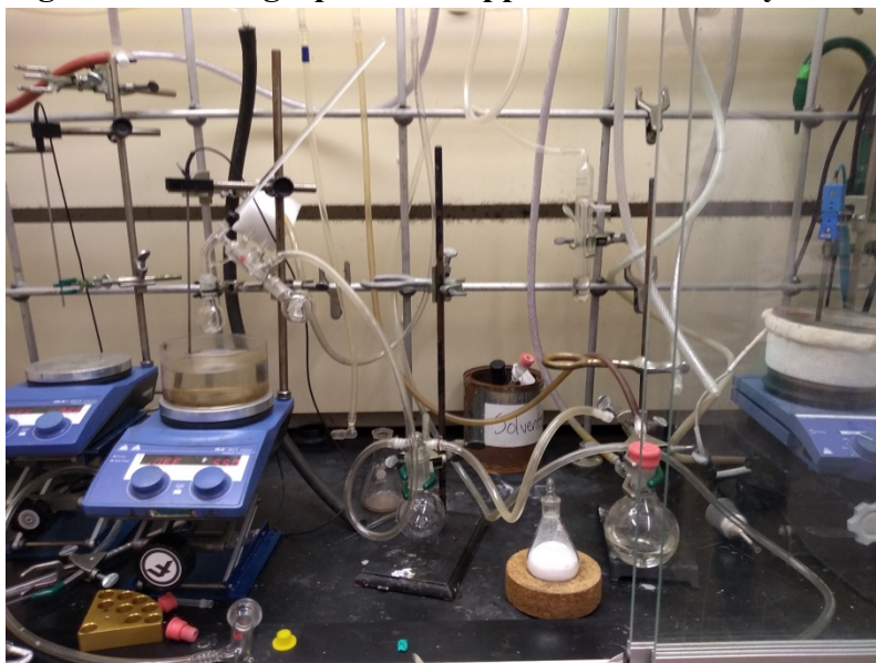
Figure E.1 Photograph of the Apparatus used to Synthesize SO 3
