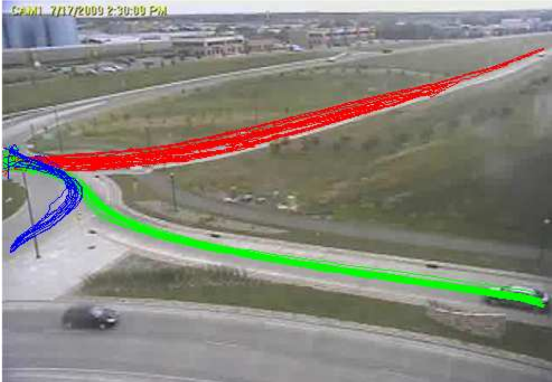
Figure 3- 3. Overlay of vehicle trajectories (one line represents one vehicle trajectory).
