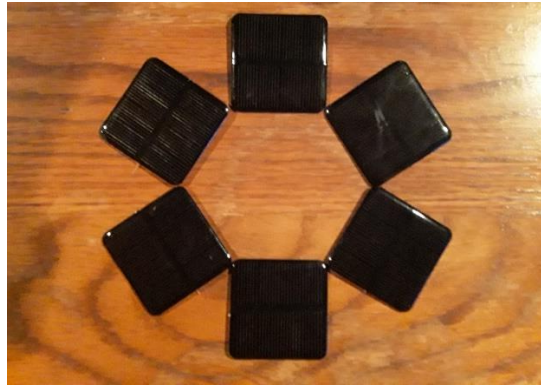
Figure 5.3: Circular pattern of PV/TEG modules used in Runs 2, 3, and 4.
