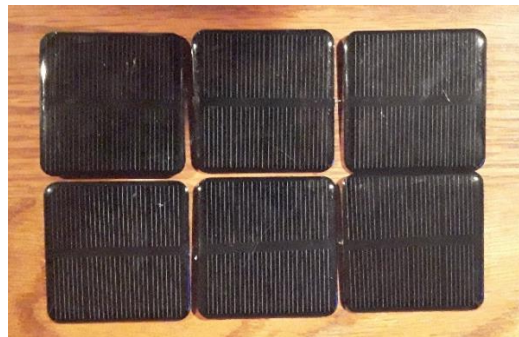
Figure 5.2: Grid pattern of PV/TEG modules used in Run 1.
