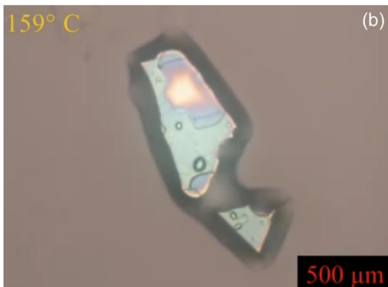
Figure 3.5 Attempt at melt crystallization for Eph-Cyc
