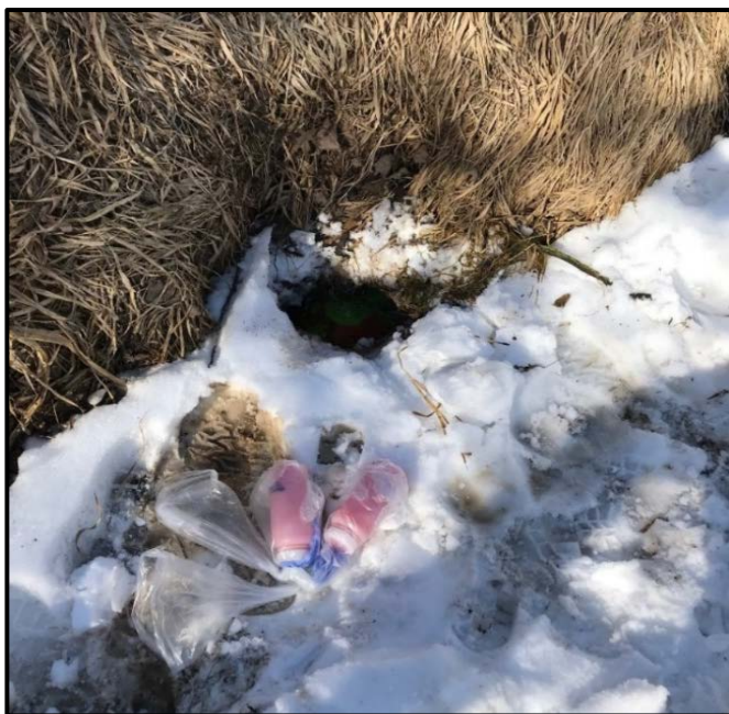
Figure 4. Dyes were poured into 23D8164 and flushed into the underlying karst system using snowmelt runoff (photo by J. Barry).
