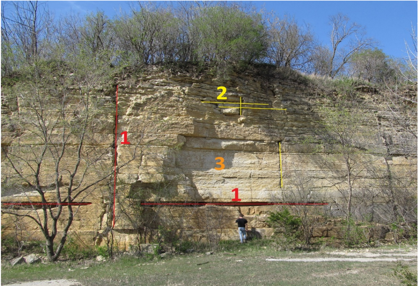
Figure 14. Prosser Formation Quarry within the Crystal Creek Watershed illustrating triple-porosity aquifer concepts. Number 1 denotes mechanical fractures and dissolution conduits that allow channel flow, number 2 denotes smaller scale fracture flow, and number 3 denotes matrix flow. Person in image is roughly 6 feet tall (photo by J.Green).
