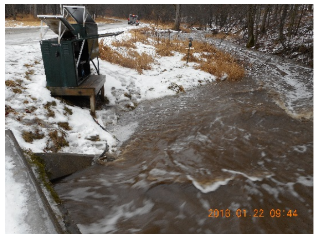
Figure 10. Flow conditions at the Crystal Creek Watershed outlet monitoring station after 1.4 inches was received on frozen soil between January 22 and January 23, 2018. (photo by C.Fischer).
