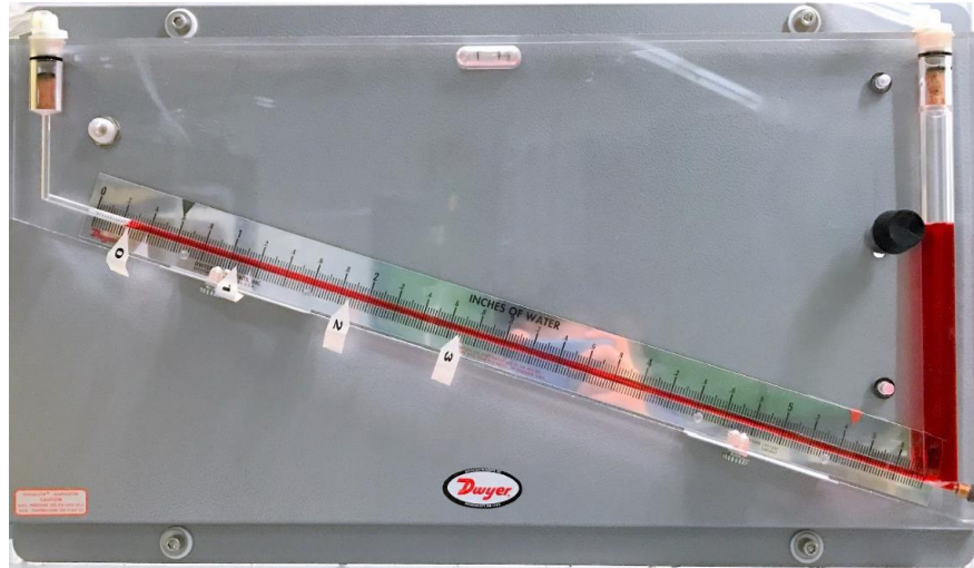
Figure 4.1: Inclined manometer used in this study (Nawathe, 2022)
