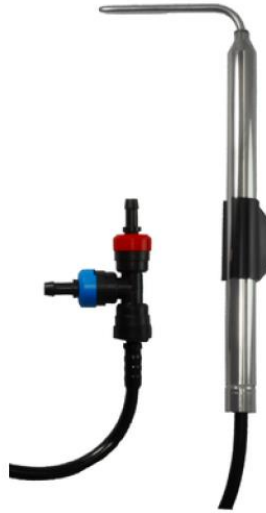
Figure 4.2: TSI Alnor Telescoping Pitot Probe. The red part is the total pressure port, and the blue part is the static pressure port. (Stinson, 2019)
