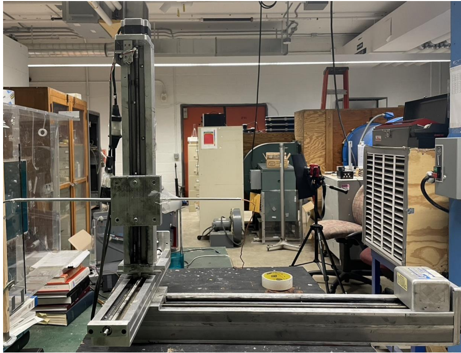
Figure 3.8: Translation device for moving the thermocouples and pitot tube probes
