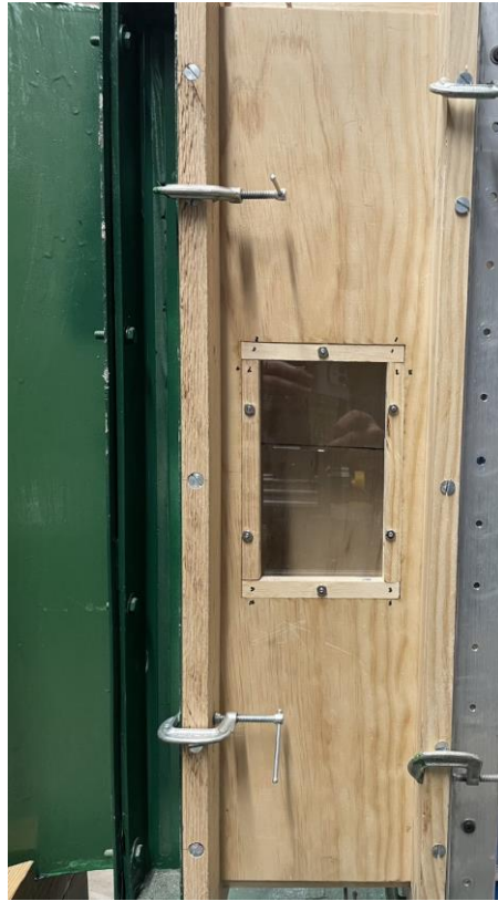
Figure 3.2: Inserted section of wind tunnel to allow flow development
