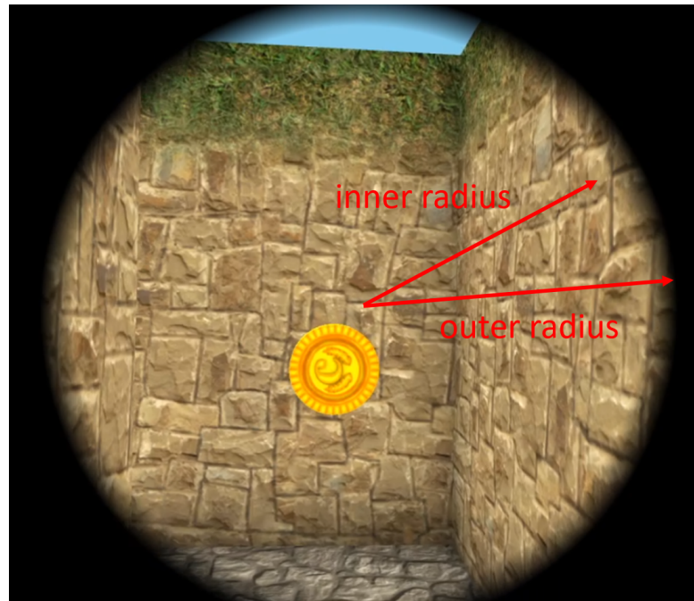
Figure 6.2: The standard symmetric FOV restriction technique uses a circular black mask to occlude the periphery. The inner and outer radii define the region in which the mask gradually transitions from fully transparent to fully opaque.
