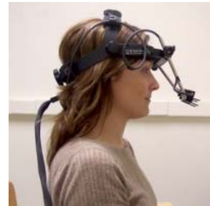
An eye-tracking helmet indicates where readers skip a word or check back in text they read on a computer screen.
