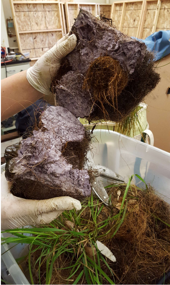
Figure 11. A root ball created by blockage of the marine-grade buoyancy foam.
