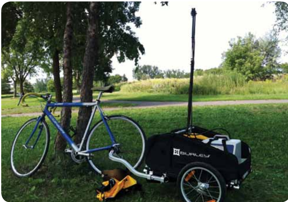
Hankey's instrumented trailer measured the air at "breathing" height rather than at tailpipe level.
