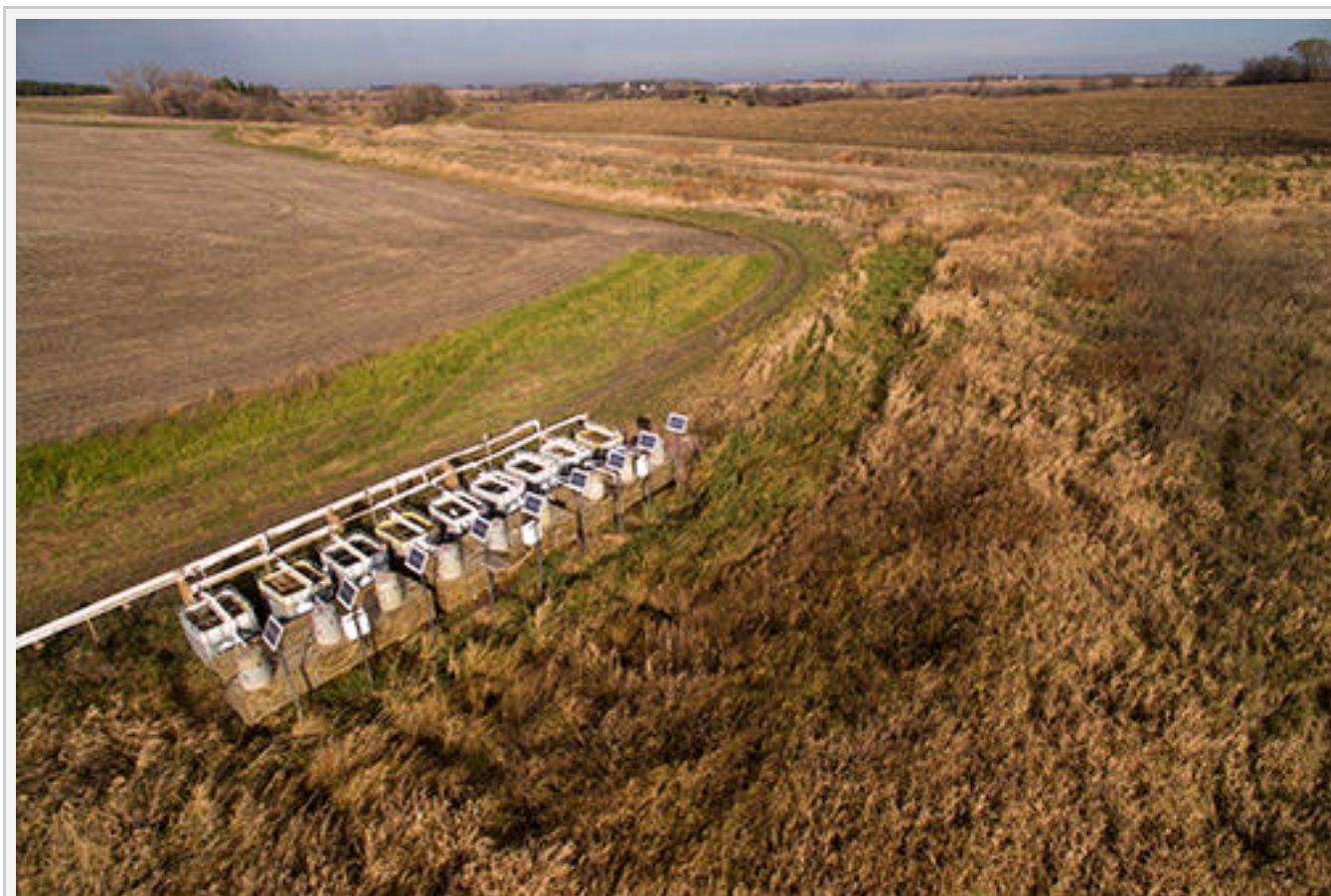
Aerial photo of the cube bioreactors. Each treatment is repeated in each block of three cubes. Each cube can nominally contain 1,000 liters of water.
