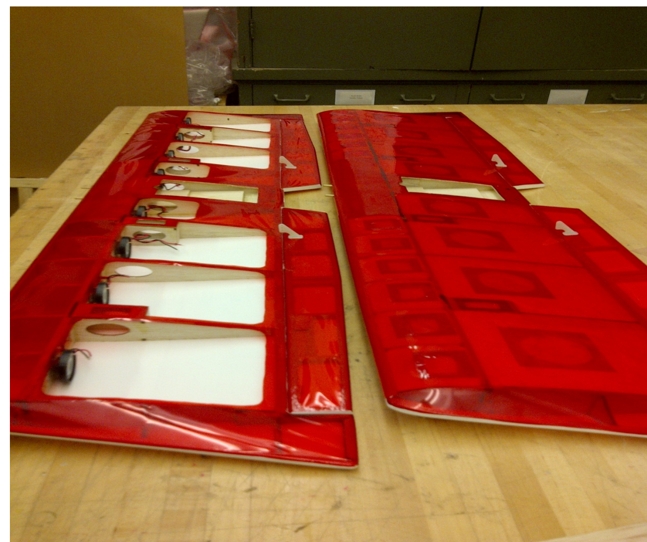
Figure 1. The Mini Ultra Stick wing filled with cotton is shown on the right. The cotton functioned to make the wing slightly solid and absorb vibrations caused by the skin. Meanwhile, the wing with mini speakers is shown on the left. The speakers are attached to the spar and being connected in series. The speakers functioned to excited small vibrations in the wing.
