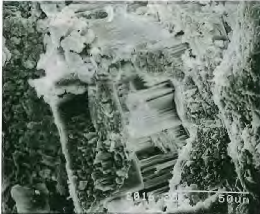
Figure 40. SEM photomicrograph of an altered orthoclase grain surrounded by kaolinite flakes. Lazear Member, Ms-1, 6.5 m.
