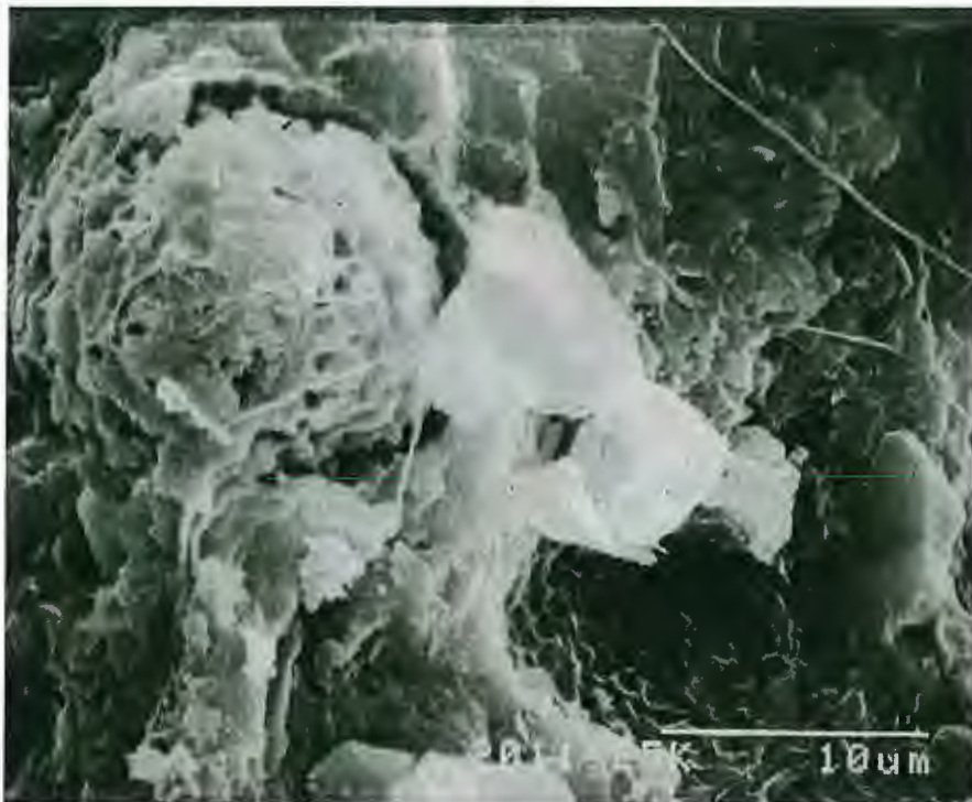
Figure 41. SEM photomicrograph of framboidal pyrite (left of center), kaolinite, smectite (elongate filaments). The sample is an interbedded shale between sand bodies of the Lazear Member.
