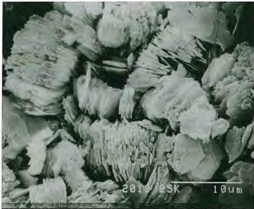
Figure 39. SEM photomicrograph of vermicular kaolinite. Lazear Member, Ms-1, 6.5 m.
