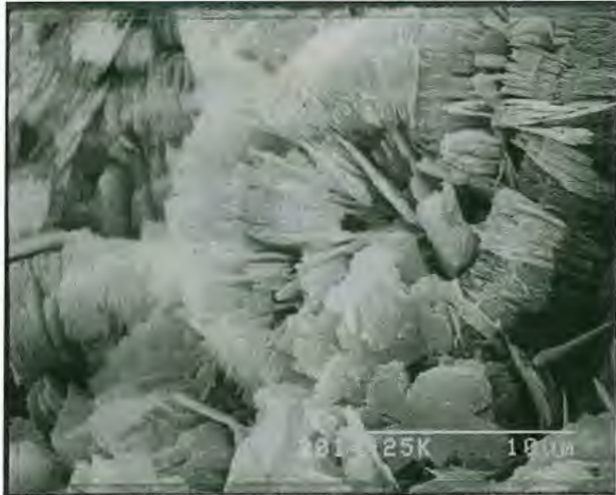
Figure 38. SEM photomicrograph of vermicular kaolinite forming delicate book structures. Lazear Member, Ms-1, 6.5 m.
