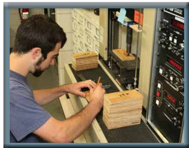
Erik Skare digitally measures the strength of wood samples. Data collected from these tests were then statistically compared to determine the best wood treatment.
