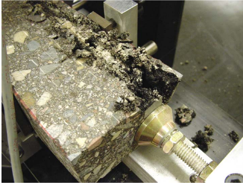
Figure 3.5. Damaged Sample after RSD Test
