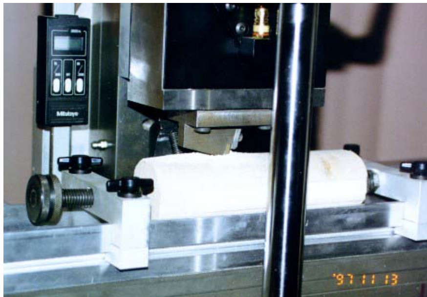
Figure 3.2. Cutting of a Rock Sample
