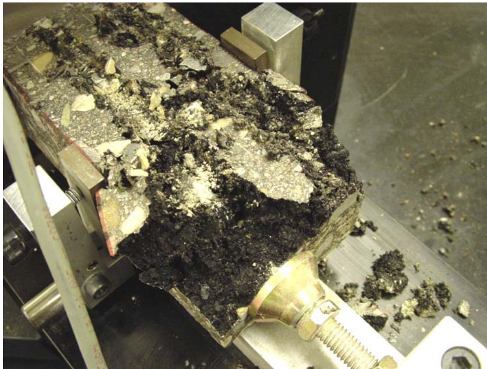
Figure 3.6. Further Destruction of Sample after RSD Test
