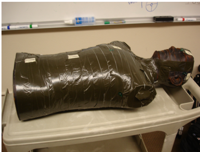
Figure 2: An anthropomorphic phantom mannequin. These are used in place of real people in radiation therapy research. A phantom’s internal electron density closely matches that of a real person.
