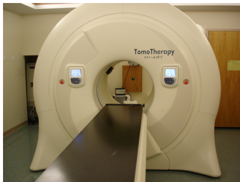
Figure 1: Helical tomotherapy treatment device. The patient lies on the platform shown, which moves in 3D through the bore, the circular enclosure that houses the radiation source. It is a largely automated procedure, but currently has no way to ensure the patients are where they are expected to be.
