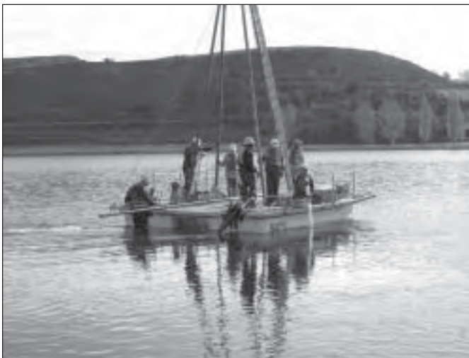
The Limnological Research Center Kullenberg coring system on Lago de Montcortés in the foothills of the Spanish Pyrenees. The expedition included Anders Noren, Doug Schnurrenberger, Penélope González, Blas Valero Garcés, Valentí Rull, Mark Shapley, and Ana Moreno. Photo by Santi Giralt. See article on page 4.
