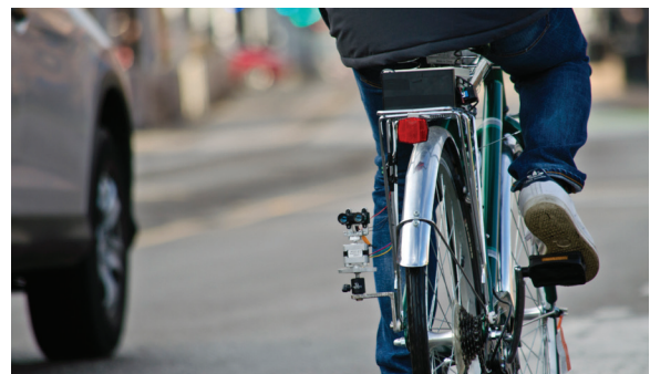
The collision-warning system uses laser sensors mounted on the bike for rear collision avoidance.
