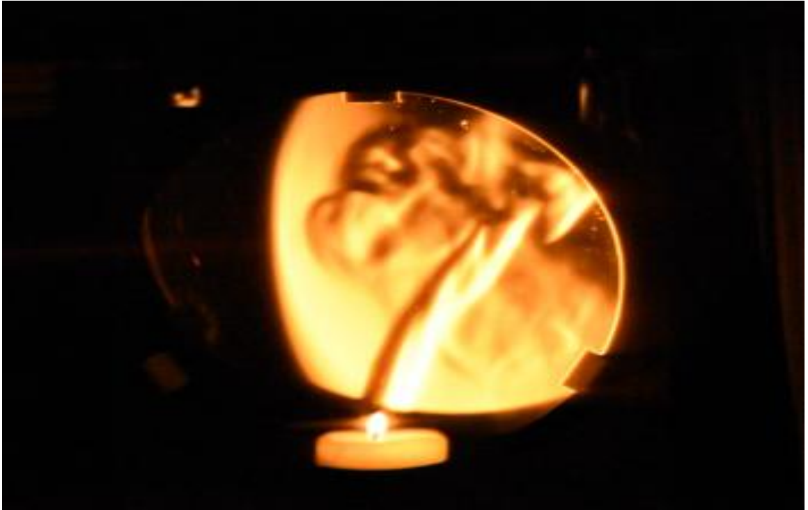
Figure 4.4 Candle Schlieren with less than 30% knife-edge
