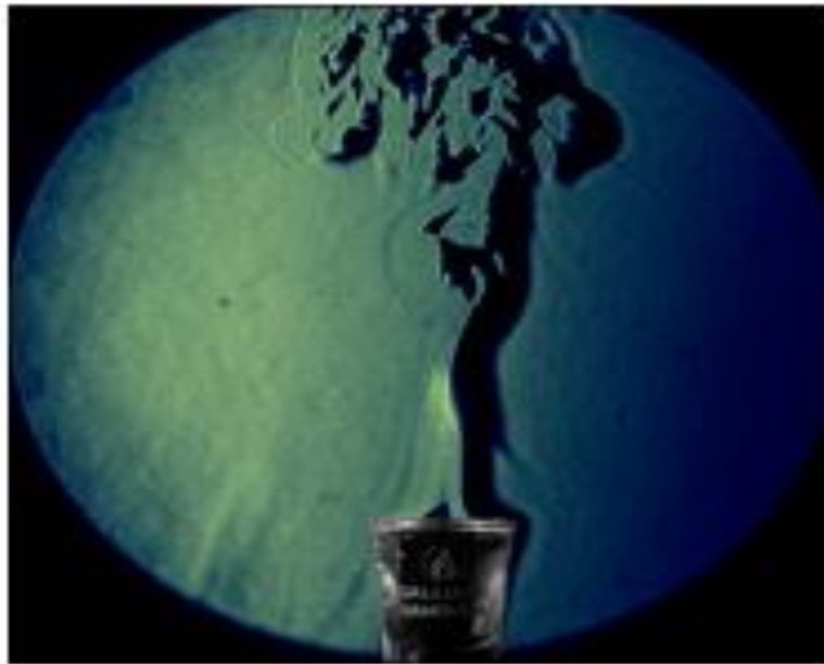
Figure 1.1: A vapor plume rises from burning alcohol. Photograph courtesy of Kasi Metcalfe [2]
