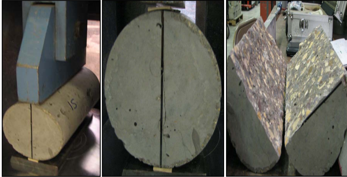
Figure D-5 Split tensile strength of concrete test setup
