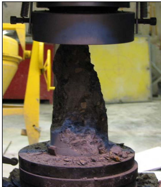
Figure D-2 Concrete compressive strength test D-9
