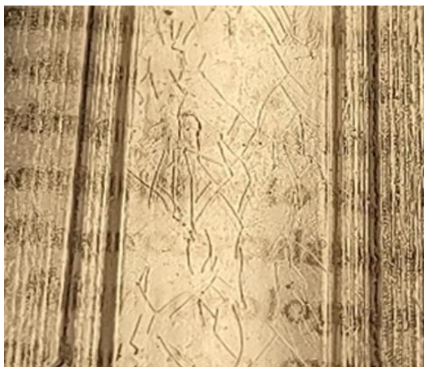
Figure 4.6 An imprinted COC wafer exposed to cyclohexane vapor for approximately 2 h. Excessive cyclohexane vapor exposure gave rise to visibly observable groove patterns in the COC wafer after solvent evaporation.
