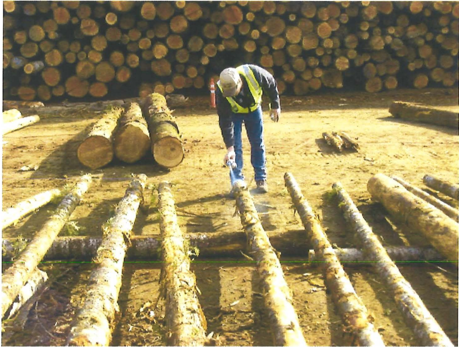
Paint stems with different colors based on acoustic velocity.
