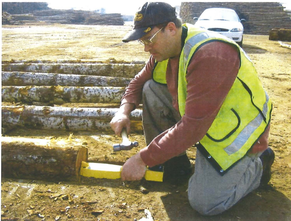
Acoustic measurement on stems.
