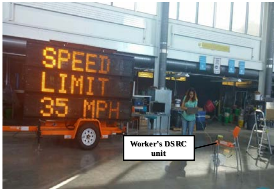
(a) DSRC unit connected to the VMS through serial connection.
