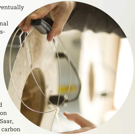
Shown above is a heater for fluid-flow and reaction experiments investigating the chemical interactions between geothermal working fluids, such as water or CO 2 , and host-rock minerals.
