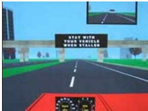
Part of the computer simulation used to test drivers' response to CMS messages.
