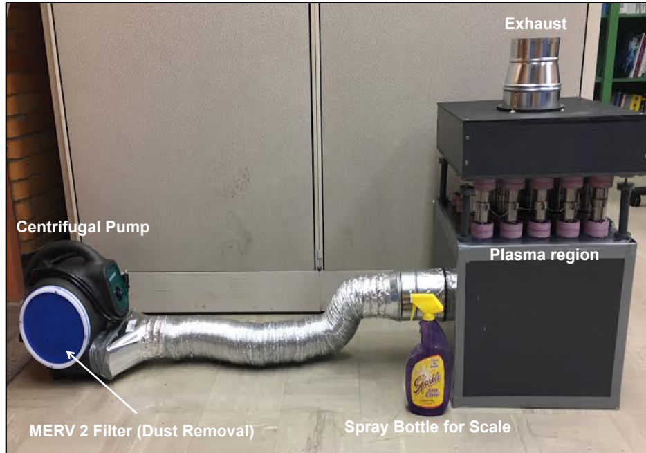
Figure 28 Pilot scale NTP system (excludes electrical equipment)
