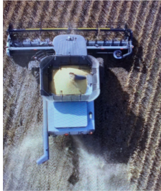
Figure 7: Uneven chaff spread pattern from combine (photo credit: Minnesota Ag Services)
