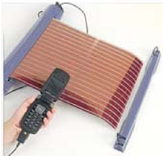
Figure 3.5. Example of a commercial organic photovoltaic module produced by Konarka Technologies that is printed on a flexible substrate. This module is being used to recharge a cellular telephone. Reproduced from Ref. 84.
