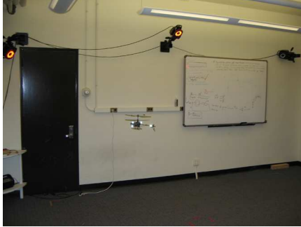
Figure 6: The experimental setup for tracking the position of the helicopter. 6 high-resolution Vicon cameras (only three shown in the picture) were placed along the perimeter of the lab that tracks the reflective markers on the helicopter (seen with bright dots in the picture) determining the position.
