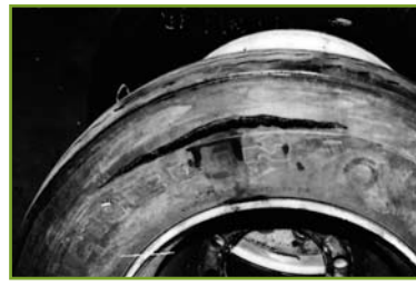
Zipper rupture on tire side wall.
