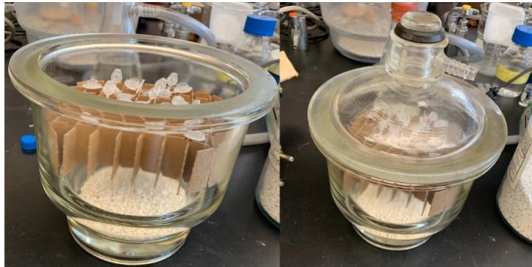
Figure 4.6.1 Desiccator with cardboard matrix and microcentrifuge tube suspension, with Drierite filled in bottom cavity. Closed and sealed on the right and open on the left.
